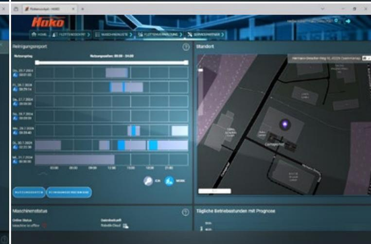
and where: the route travelled by the machine (municipal technology) can be tracked precisely using an interactive map.
